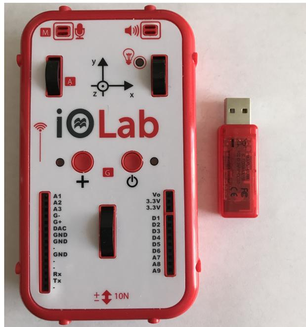
Figure 1: The primary contents of the iOLab device. From left to right, the device/remote and the Dongle.
