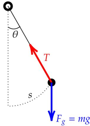
Figure 5.1: Forces acting on the point mass in a simple pendulum.
