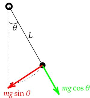
Figure 5.2: Components of the gravitational force acting on the point mass.
